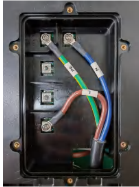
Cable harness diagram FEV-T16/32 (1Ph Connection guide)
