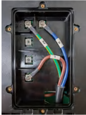
Cable harness diagram FEV-T16/32 (1Ph Connection guide)
