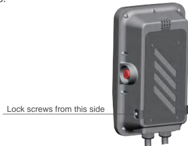
Charger box locking on back plate diagram
