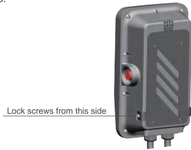
Charger box locking on back plate diagram
